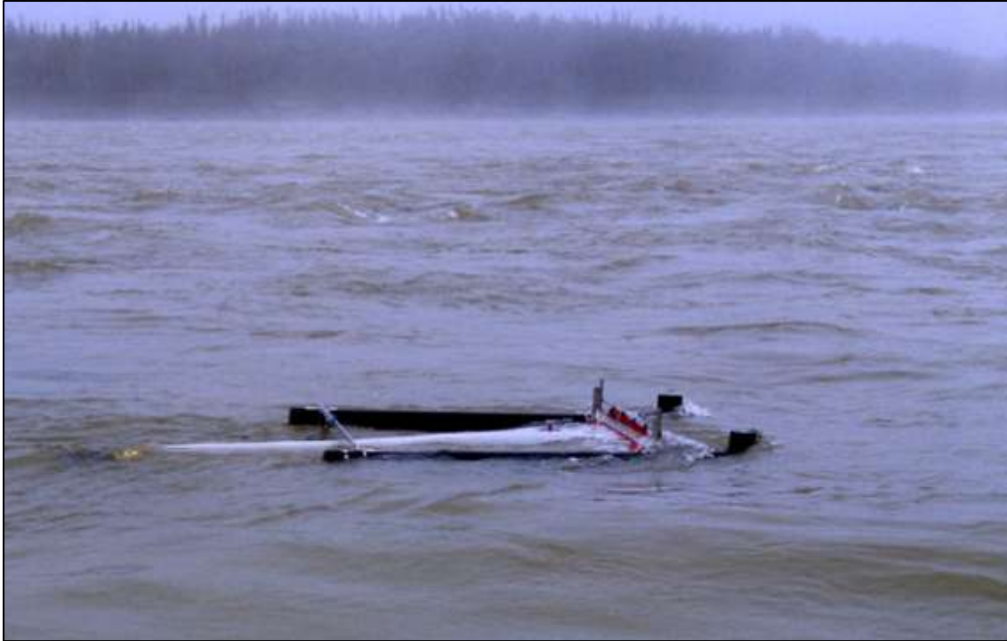
Photo 6B-2: Floating drift trap used to capture newly-hatched larval lake sturgeon as they drift downstream in the Keeyask study area
