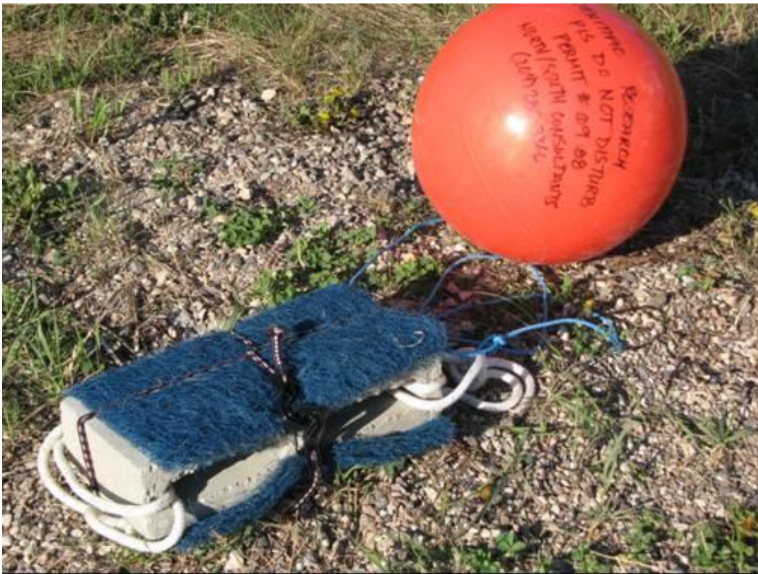
Figure 10. Egg collection mat used to monitor spawning on and near the constructed shoals.
