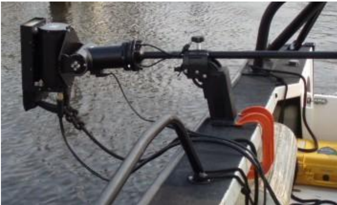
Figure 11. DIDSON acoustic camera and pole mount used to monitor the constructed shoals.
