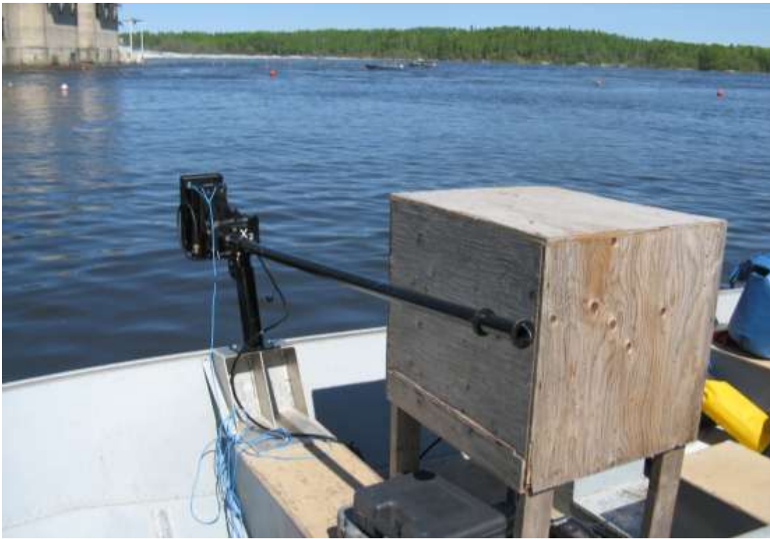
Figure 3. DIDSON acoustic camera and pole mount used to monitor the constructed shoals.
