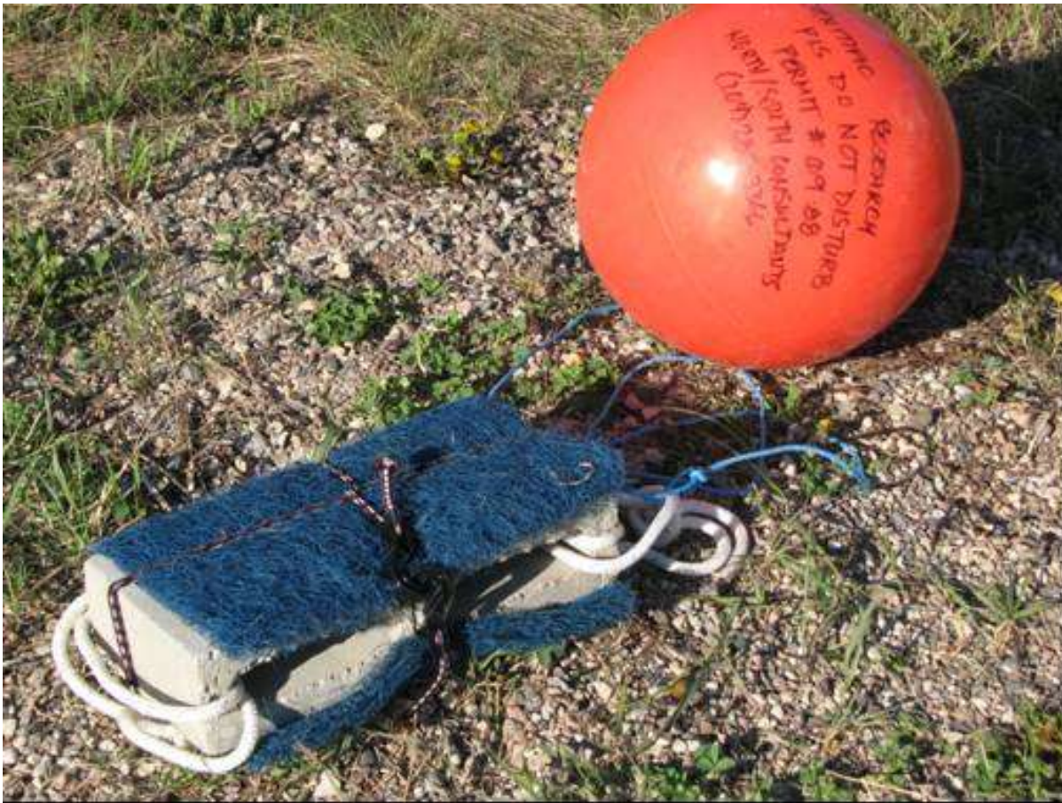
Figure 7. Egg collection mat used to monitor spawning on and near the constructed shoals.
