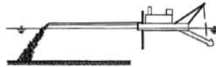
Surface Discharge with Pipeline
