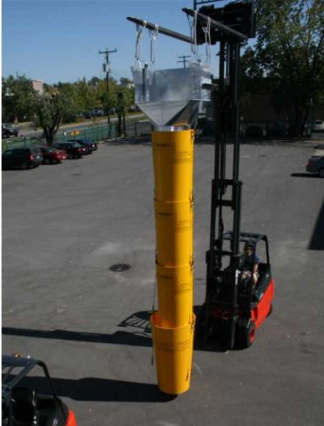
Photo 1 Keyask GS, Stage IV Studies – Axis GR-4 Example of Retractable Plastic Chute with Hopper
