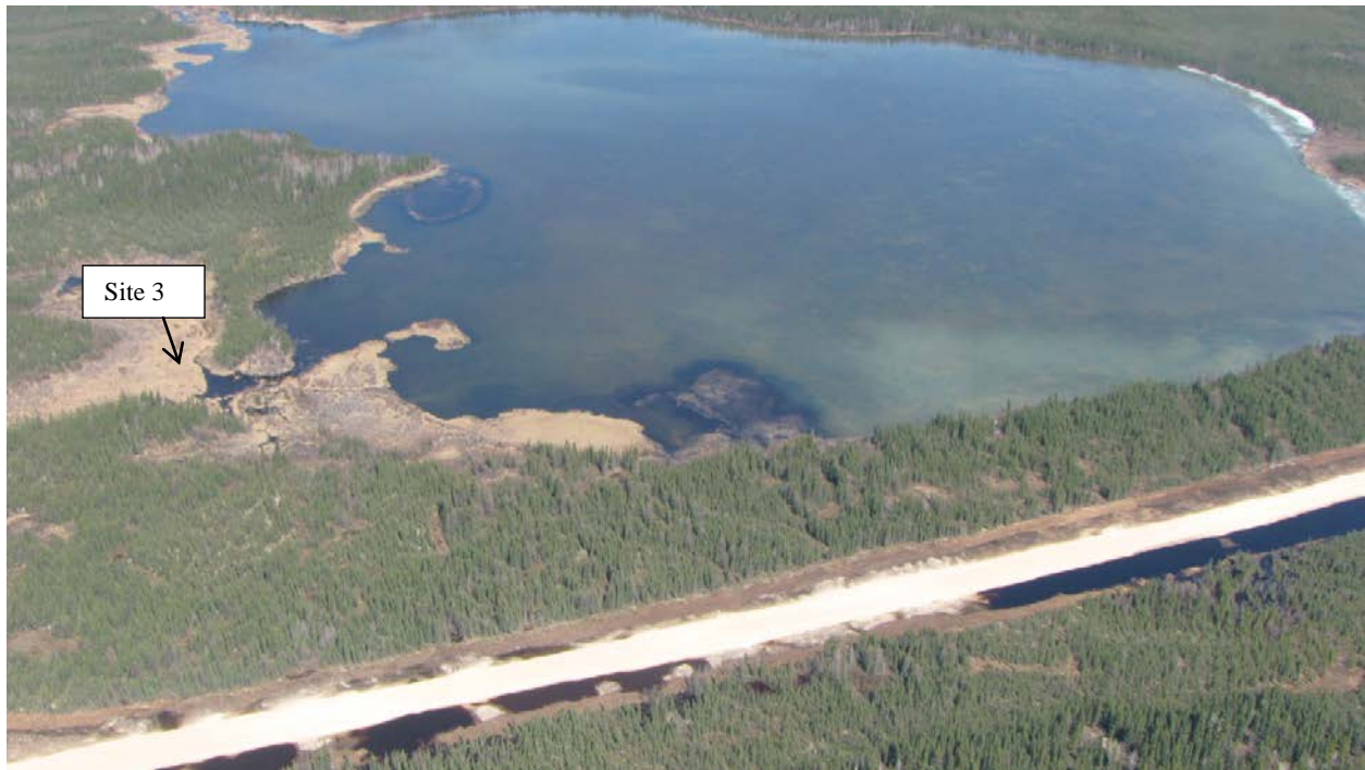
Photo 3-3: Ponding of Water Along the KIP Road near Site 3 (May 2012).
