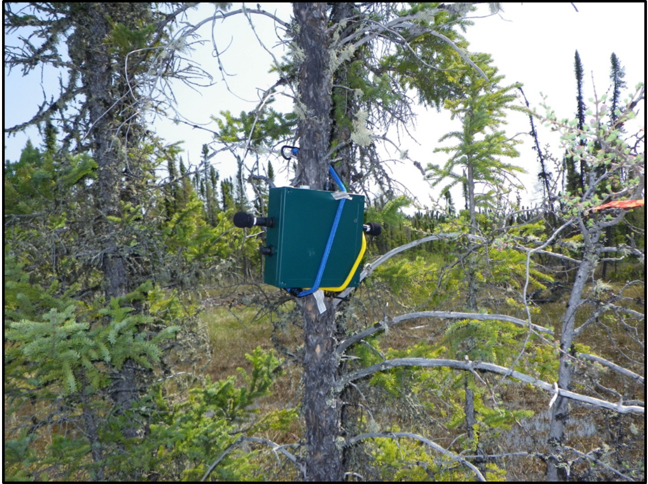
Photo D-2: Remote Recorder Unit Set-up
