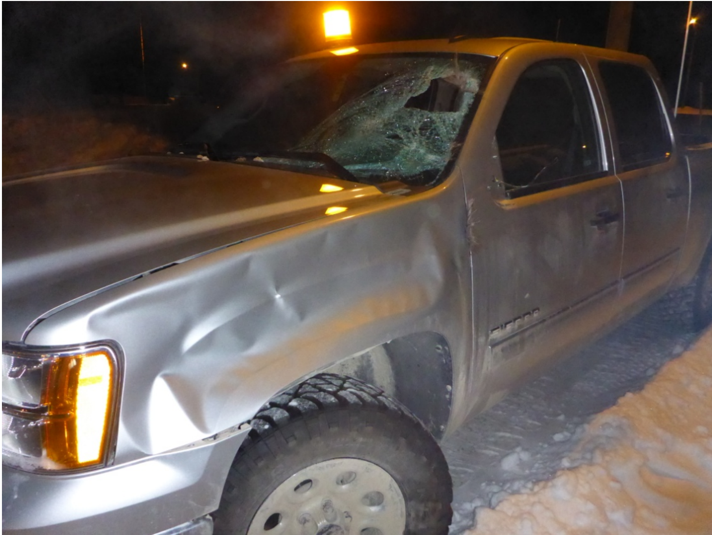
Photo D-5. Truck damage after a moose collision at Kilometre 11 of the access road on November 18, 2013.
