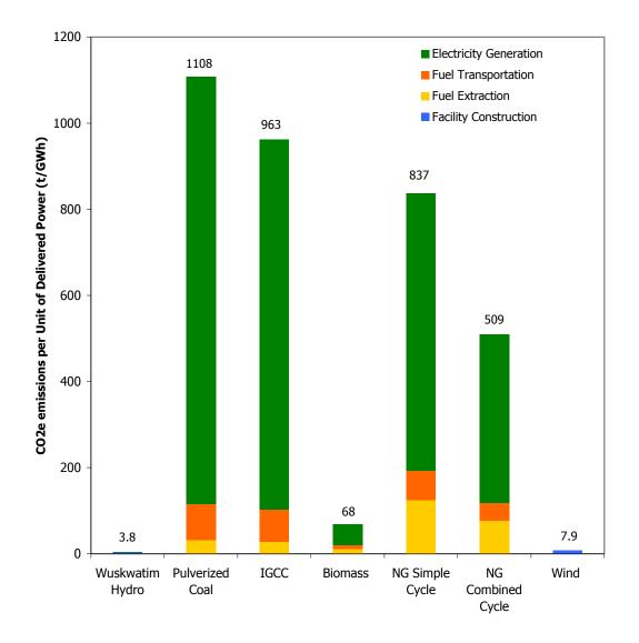
Figure 3.1 Life Cycle GHG Emissions per Unit of Delivered Power for Each Electricity Supply Option
