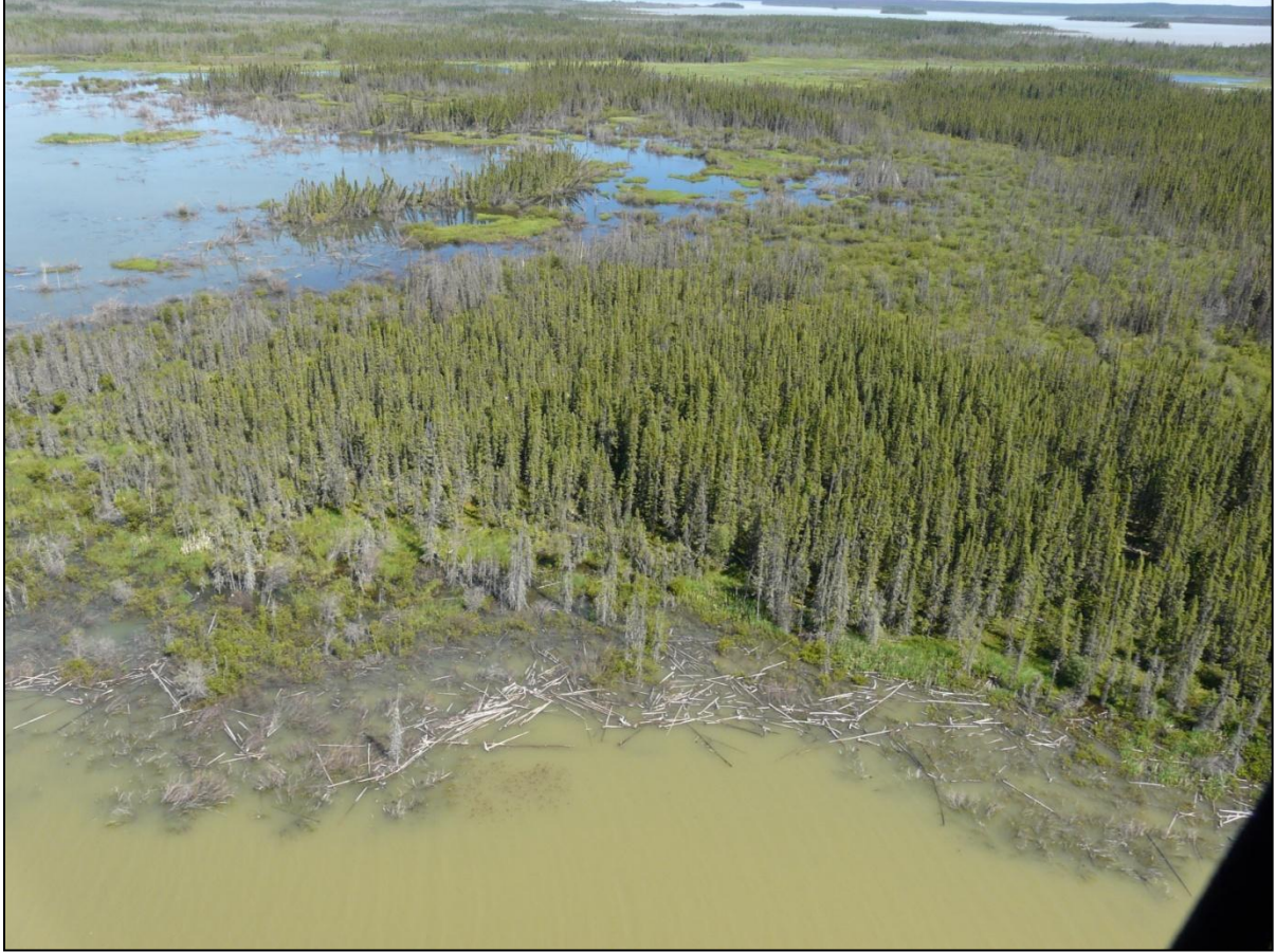
Photo 6-11: Searched shoreline in the western portion of the Kettle reservoir showing shoreline recession due to peatland disintegration, tree mortality and composition change in the shore zone between 1971 and 2003/2006. Photo taken in 2011, looking northwest (Map 6-4)
