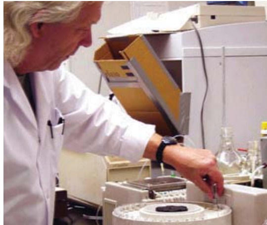
Researcher placing digested muscle sample into mercury auto-analyzer.
