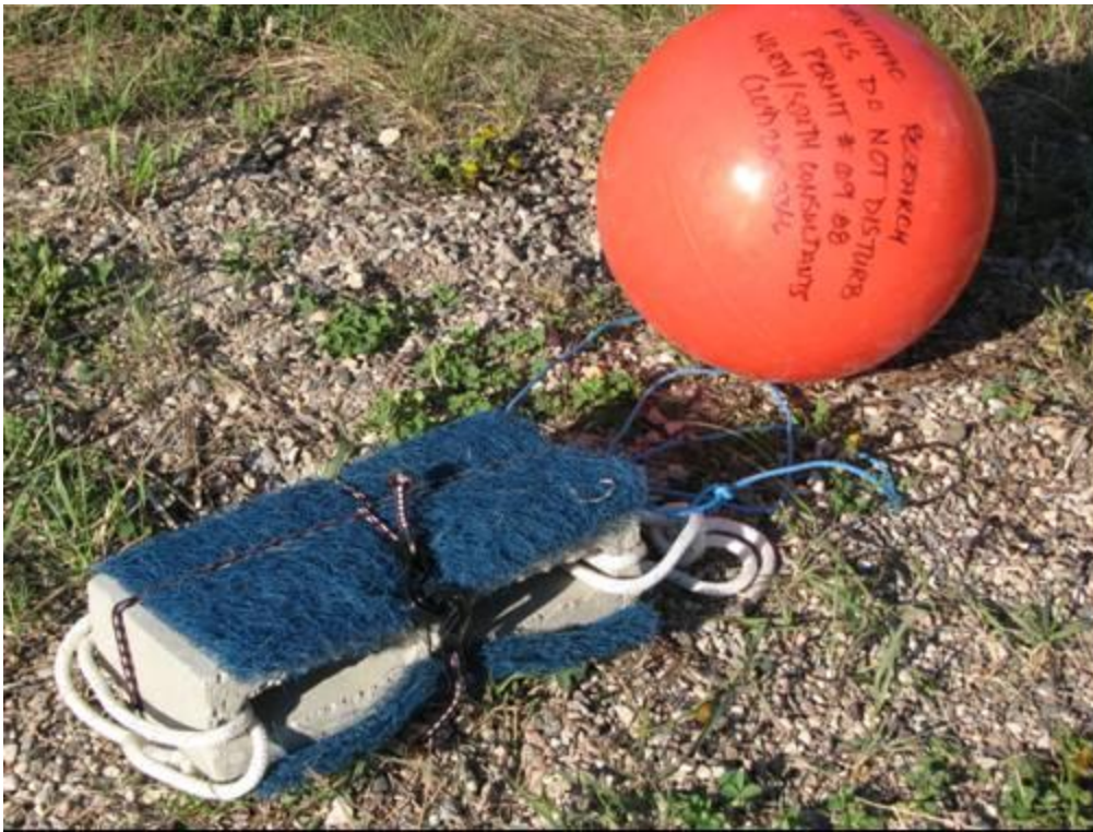
Figure 4. Egg collection mat device used to monitor spawning on and near the enhanced spawning ground.
