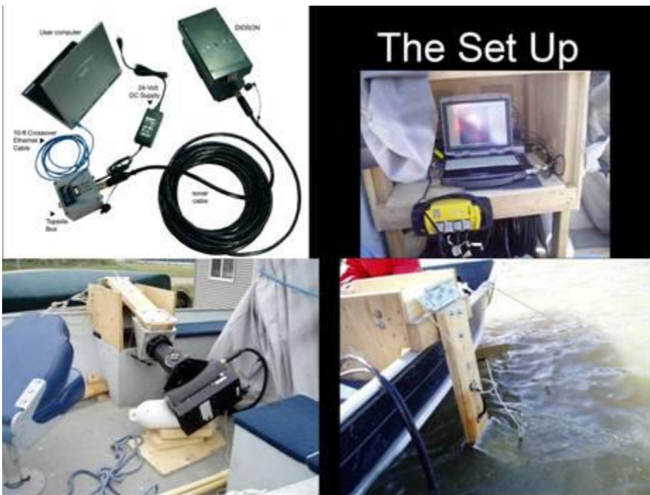
Figure 5. Didson sonar camera set up used to monitor the enhanced spawning ground.
