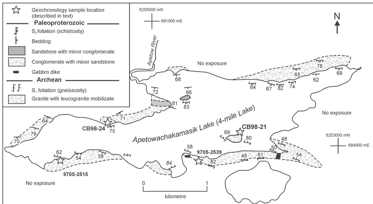
**Figure GS-7-2:** Simplified geology of Apetowachakamasik Lake.
