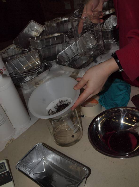
Figure 4 – Filtering the floating material removed with a porous scoop.
