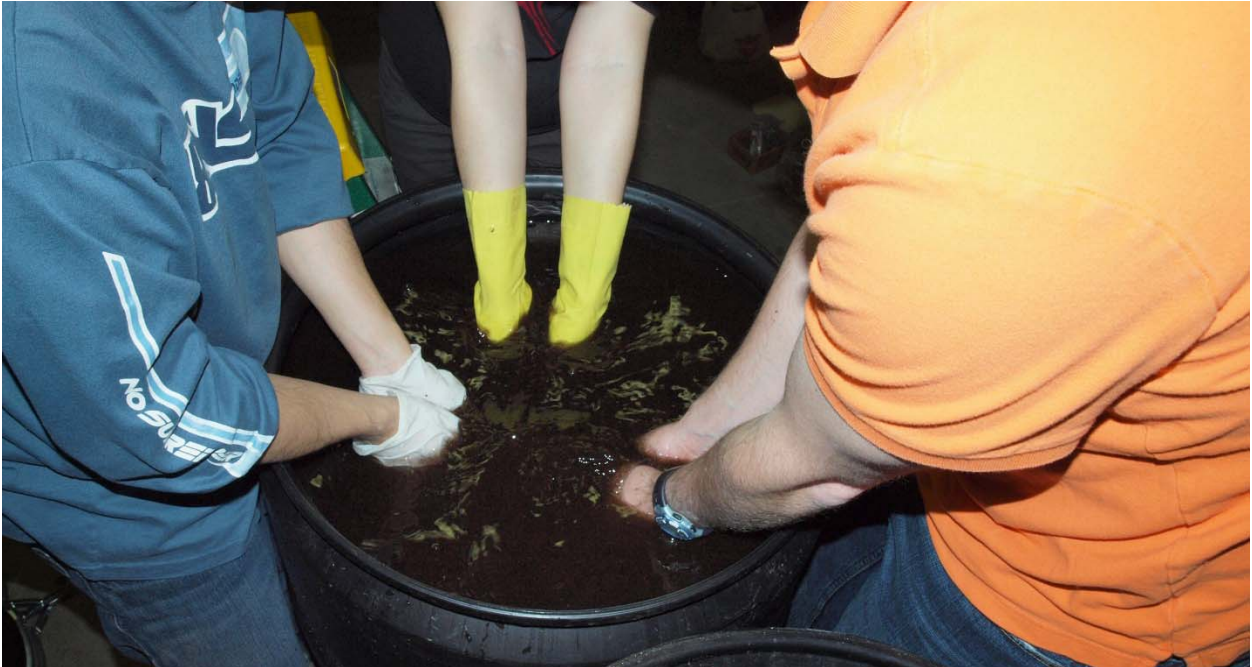
Figure 3 – Hand agitation of peat samples.
