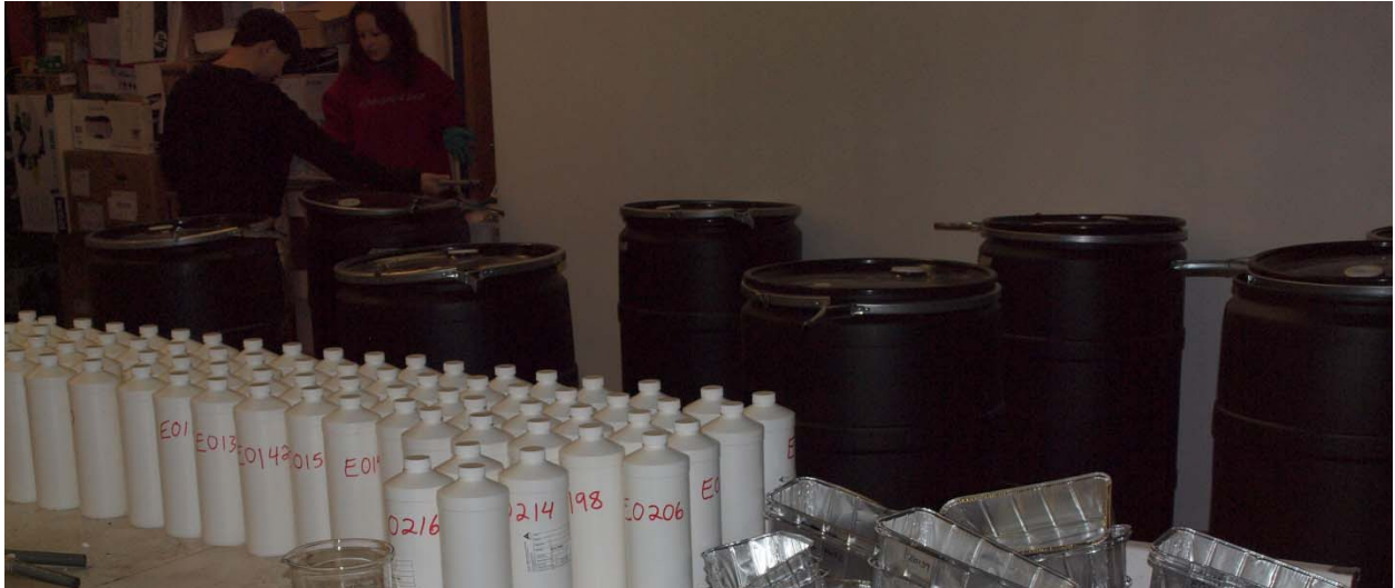
Figure 2 – Barrels next to the wall being filled with water. Bottles for TSS-analysis and containers for oven-drying are in the foreground.
