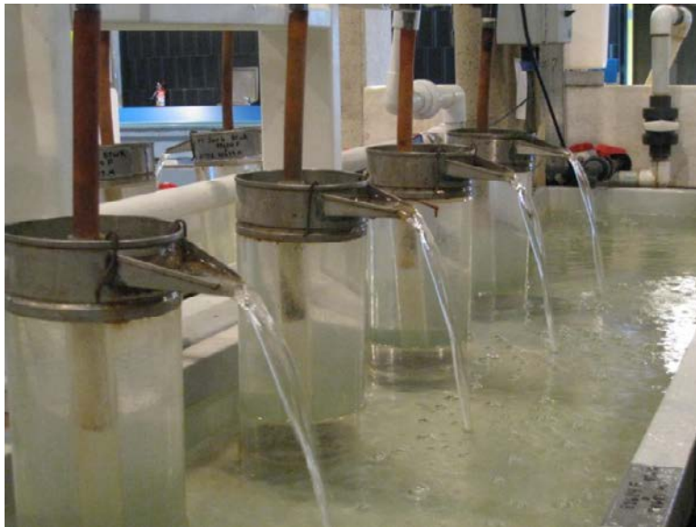
Figure 2: McDonald hatching jars used to incubate lake sturgeon eggs
