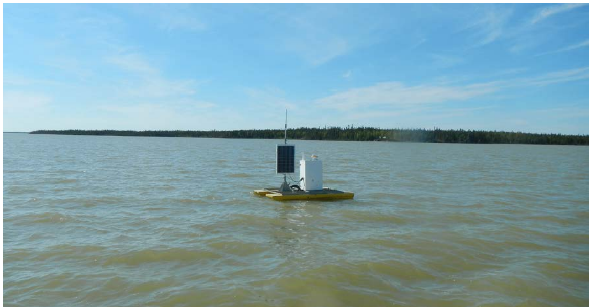
Photo 6: Installing Turbidity Monitoring Equipment and a Station after Installation
