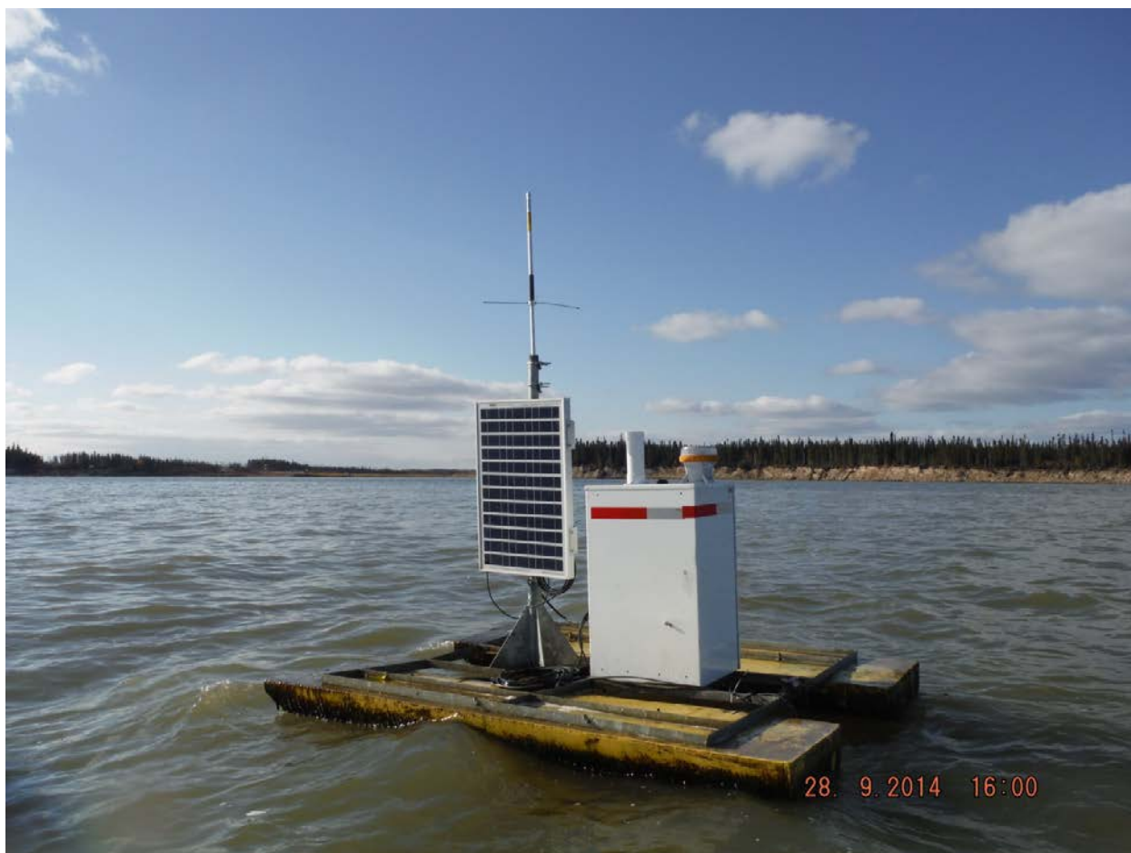
Continuous turbidity monitoring site – turbidity sensors suspended below catamaran that supports solar power panel and electronics housing
