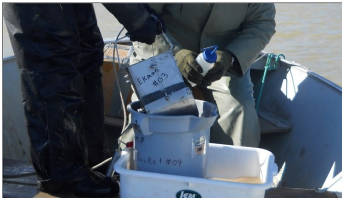
Collecting a benthic macroinvertebrate grab with an Ekman dredge
