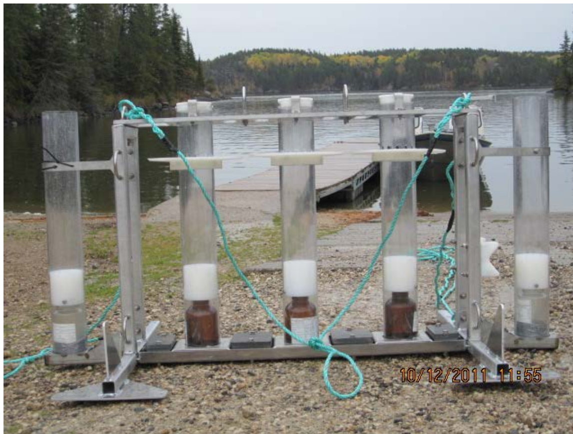
Five tube sediment trap used in PEMP deposition monitoring
