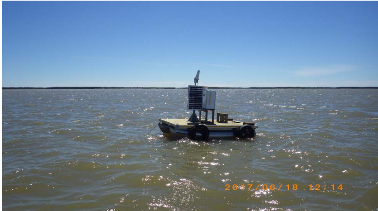
Continuous turbidity monitoring equipment – electronics cabinet and solar panel on a catamaran below which a turbidity sensor is suspended in the water
