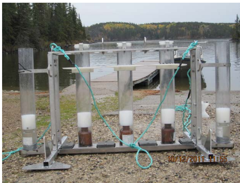
Photo 6: 5-Tube sediment trap used at site K-ST-02
