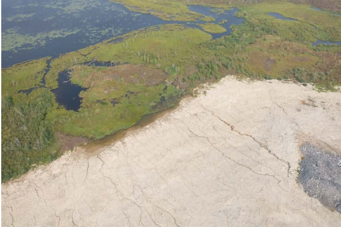
Aerial view of EMPA slope near the east shore of Wetland 51, showing erosion channels and sediment entering marsh habitat buffer
