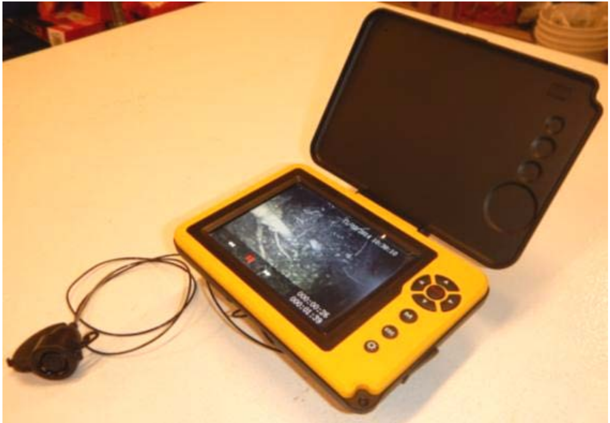
Figure 2-1: Aqua View Micro 5 Camera with Built-in Digital Video Recording and Infrared Light Source, Used to Confirm Den Occupation
