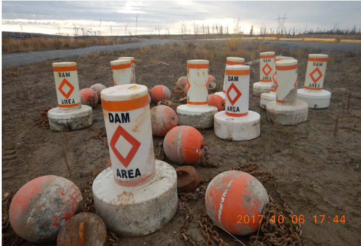
Figure 7: Warning buoys that are deployed downstream of Gull Rapids during the open-water season were removed for winter storage and were visually inspected for the presence of adult and juvenile zebra mussels
