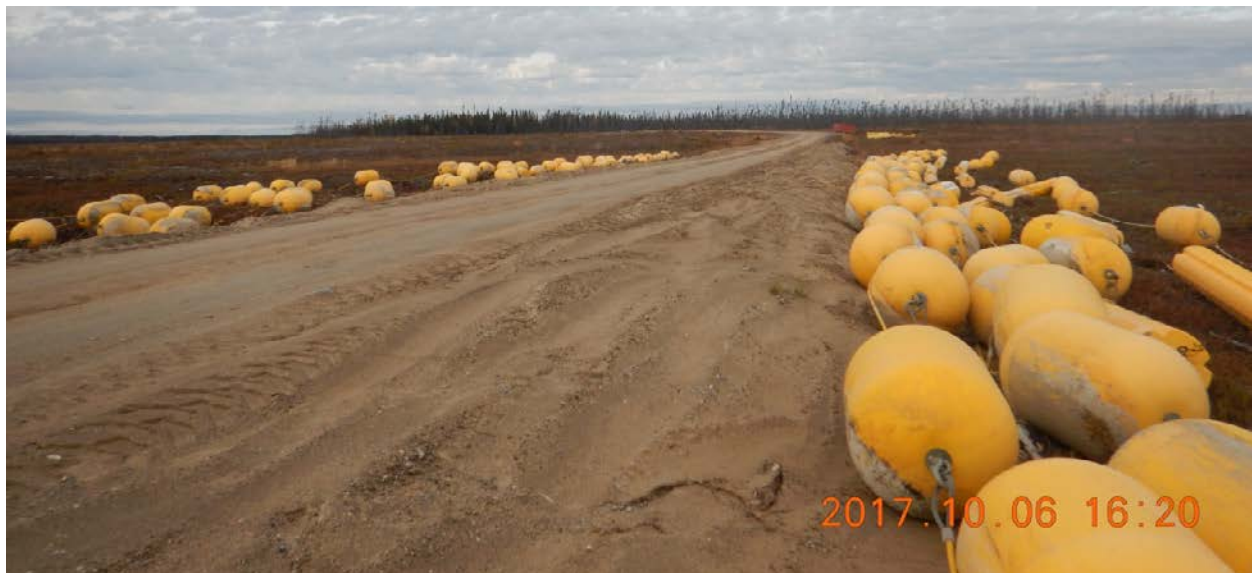
Figure 6: Parts of the open-water safety boom that had been removed for winter storage were visually inspected for the presence of adult and juvenile zebra mussels
