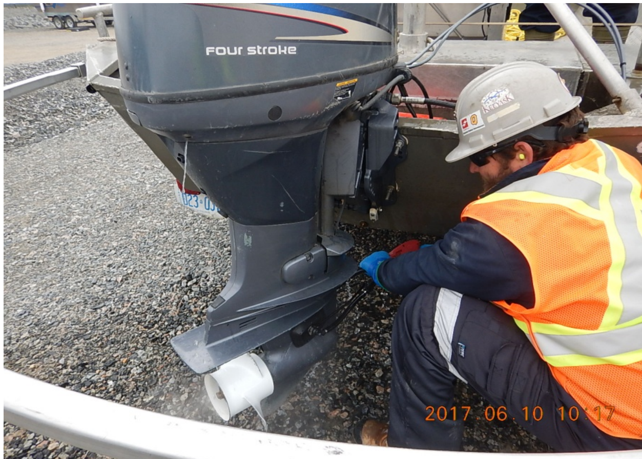
Figure 1: A boat motor being decontaminated by flushing with hot water ( \geq 60 °C) on June 10, 2017
