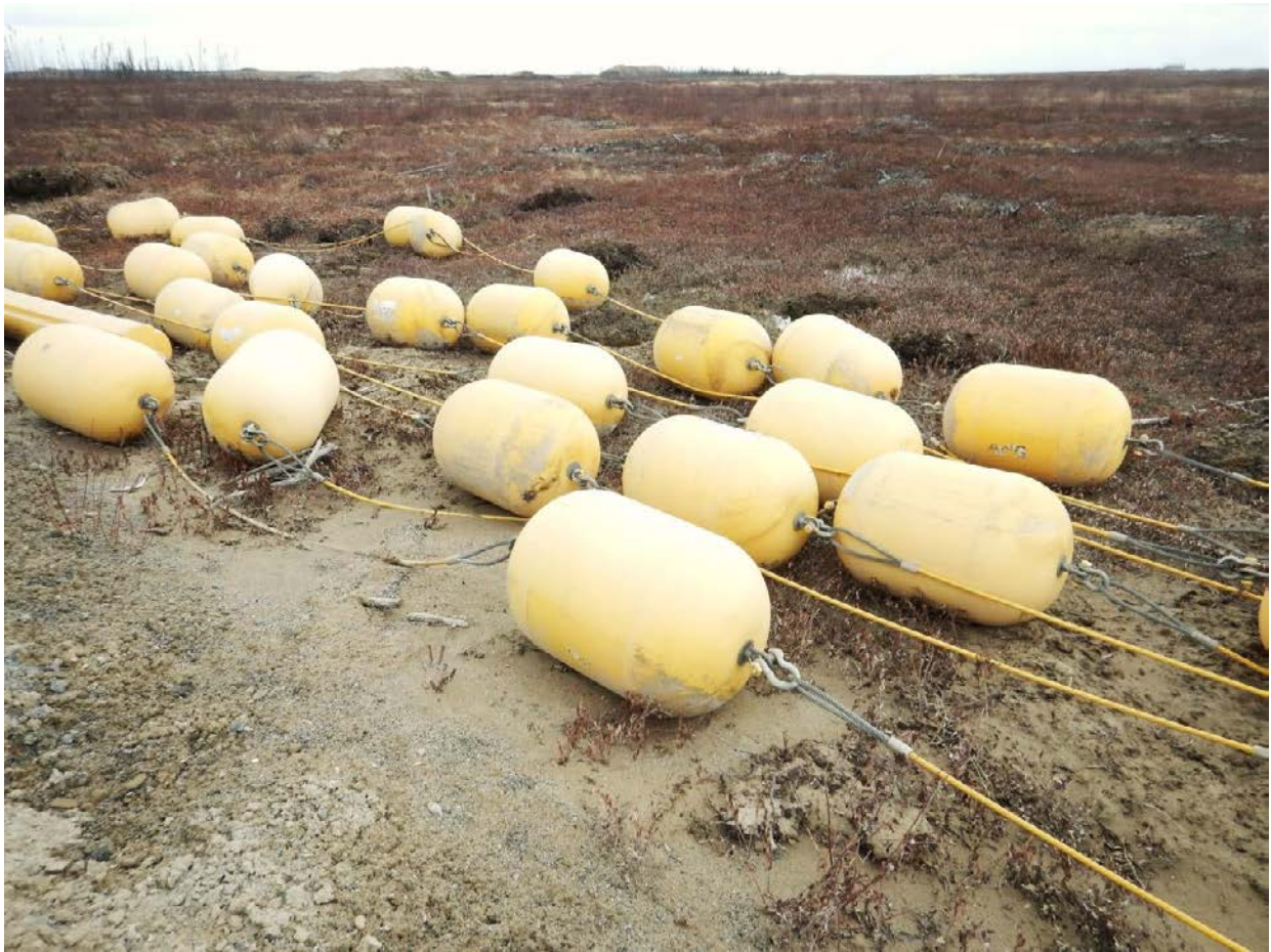
Photo 5: Parts of the open-water safety boom that had been removed for winter storage were visually inspected for the presence of adult and juvenile zebra mussels
