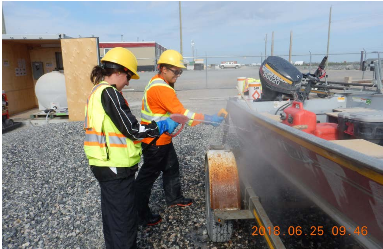
Photo 2: A boat being decontaminated by rinsing with hot water ( \geq 60^{\circ}\text{C} ) on June 25, 2018
