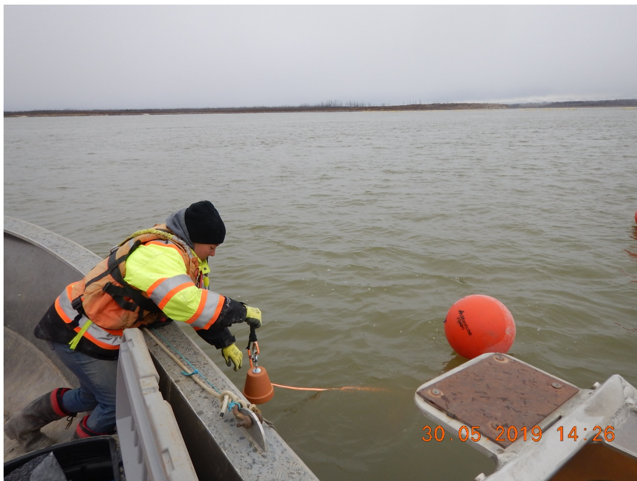
Figure 6: Installing artificial substrate to monitoring for zebra mussel colonization, May 30, 2019.
