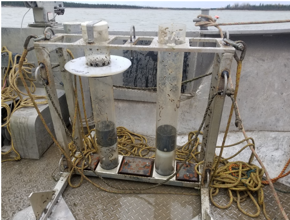
Photo 11: Sediment traps - 2 tube design
