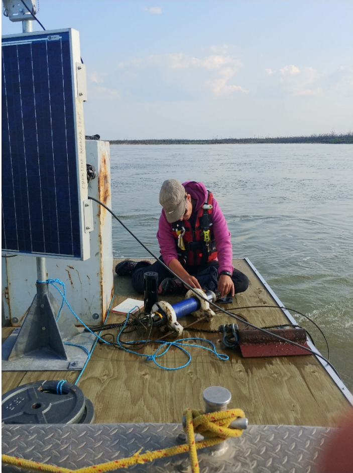
Continuous turbidity monitoring equipment – setting up a turbidity sensor
