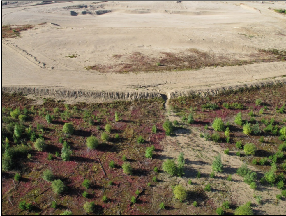
Photo 3-4: Erosion and sediment deposition at northern edge of Borrow Area G-1 at KM 17
