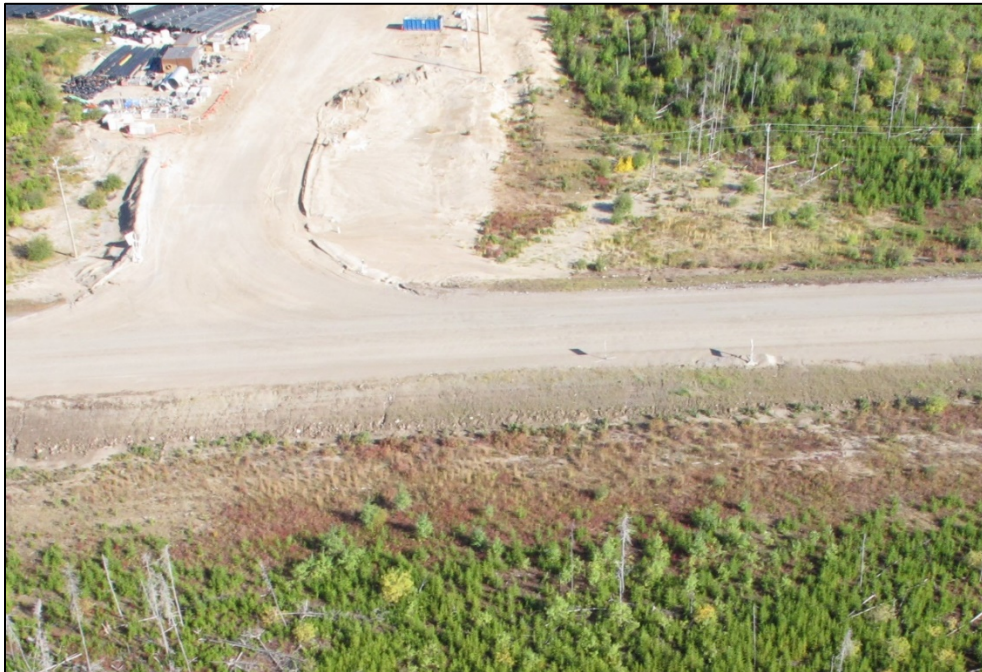
Photo 3-5: Sediment deposition at entrance of Borrow Area G-1 at KM 17
