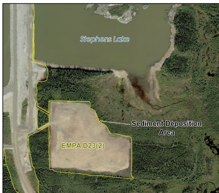
Figure 3-4: Erosion and sediment deposition from EMPA D23(2)-E
