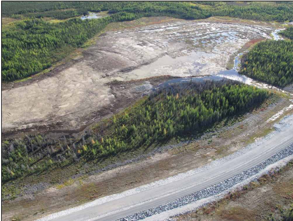
Photo 3-21: Aerial view of ponded water and dying trees on northern edge of EMPA D27(4)
