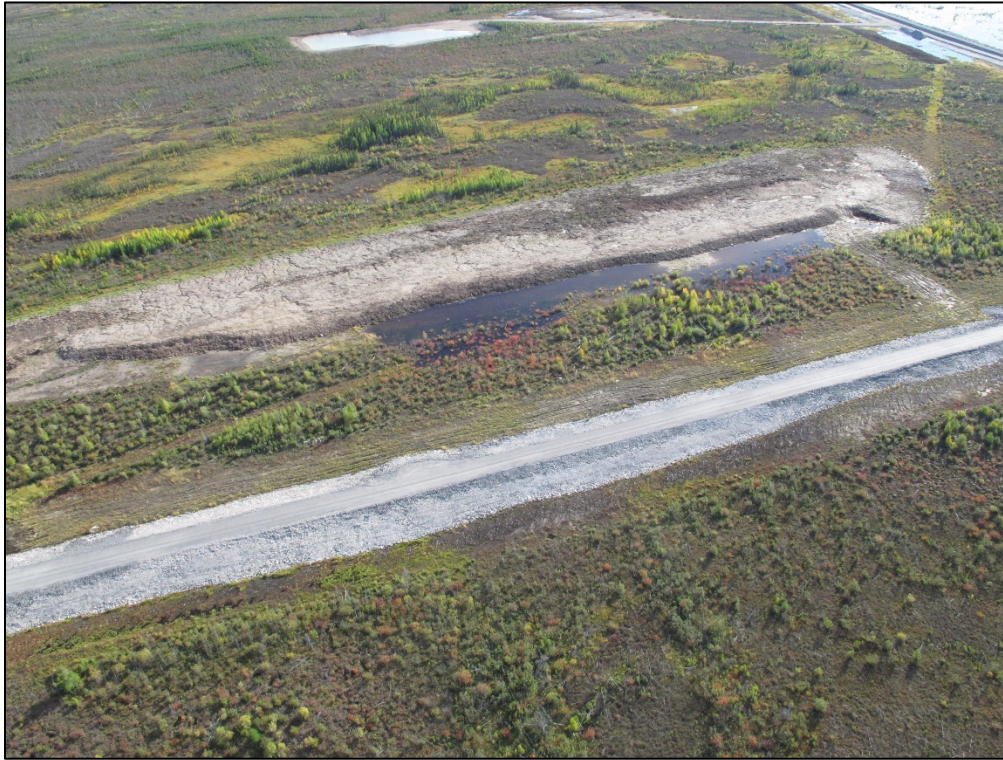
Photo 3-22: Aerial view of ponded water and dying vegetation on northern edge of EMPA D28(1)-E
