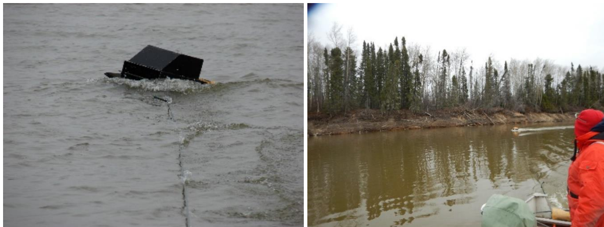
Neuston sampler (left), towed behind boat (right) to capture Lake Whitefish larvae drifting in the water column after hatch.
