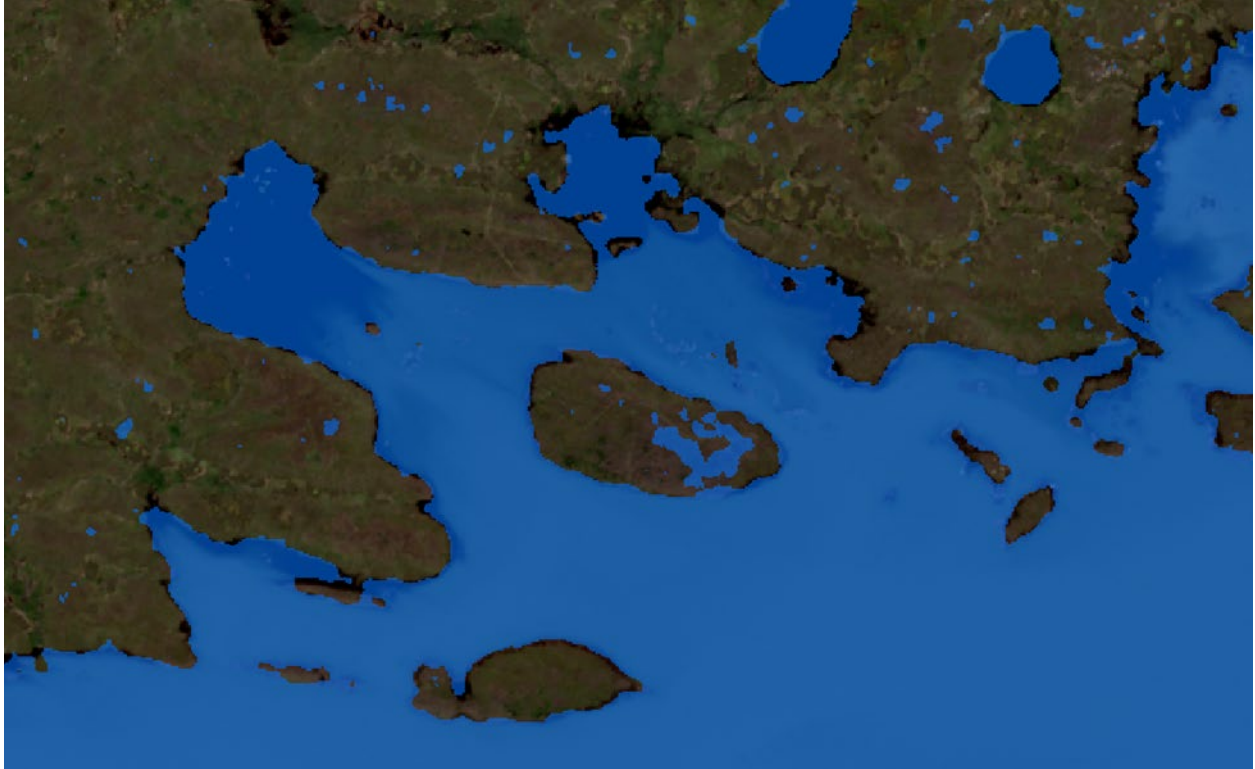
Figure 2: Image of SAR June 12, 2021 threshold value of -18.5 dB used to discriminate water (blue) from land (June 14, 2021 Sentinel-2 image in background) in the Keeyask GS reservoir near the Hidden Creek (MS7) nearshore monitoring site. Note that the method often underestimates open water extent closer to shore, while overestimating water over floating peat, debris, and wetland targets likely saturated with water.
