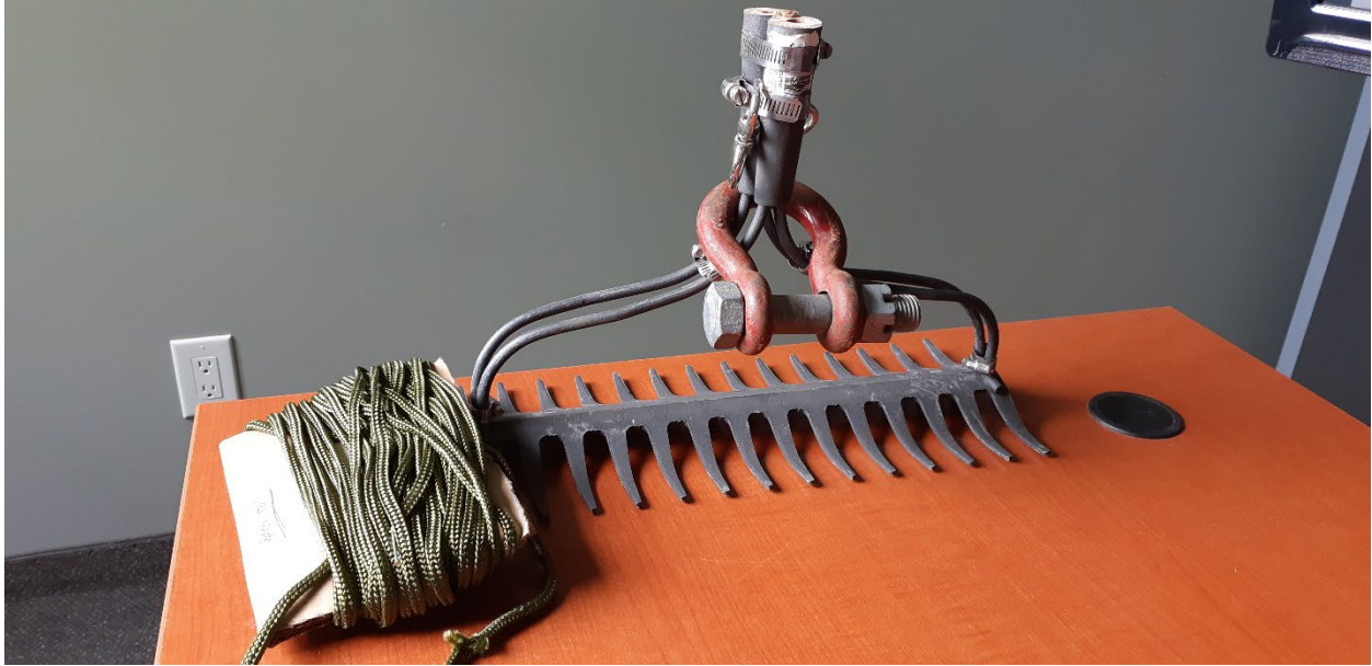
Photo 1: Image of the weighted double headed rake sampler.
