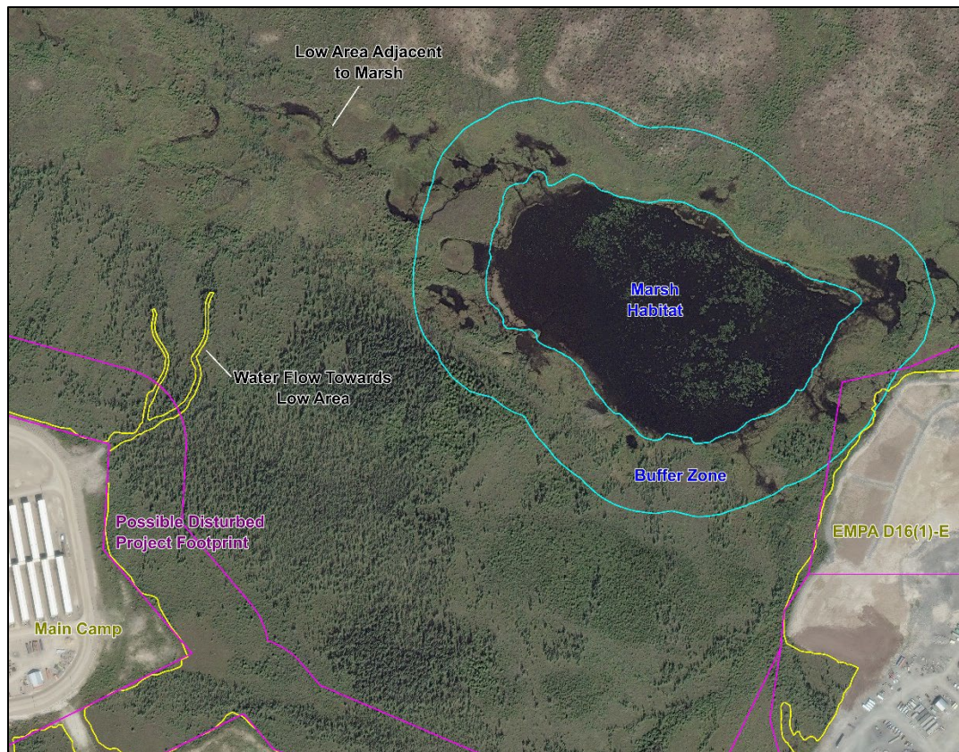
Figure 3-13: Extent of water flow from culvert (in yellow to the west) with potential to affect Wetland 51 (in blue) as of September, 2021
