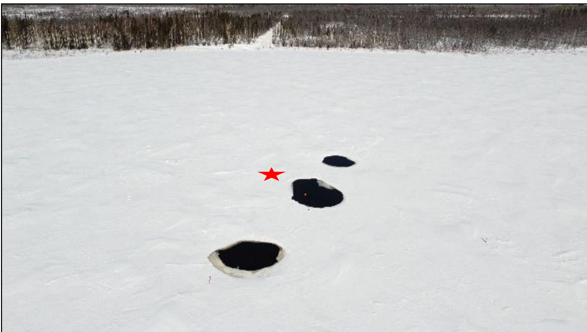
Image showing where the dissolved oxygen meter was installed during winter 2021/2022 (indicated by the star) and areas near the aeration system that remained ice-free all winter.
