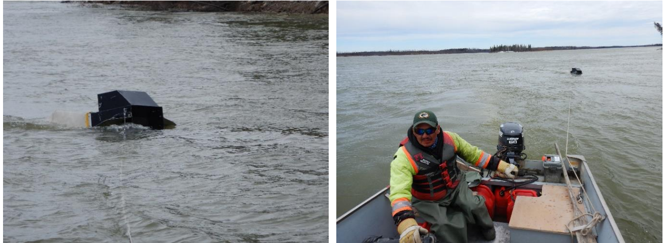
Neuston sampler (left), towed behind boat (right) to capture Lake Whitefish larvae drifting in at the surface of the water column after hatch.
