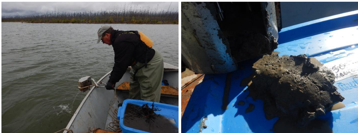
Collecting substrate (right) at a benthic invertebrate sampling site with a petite Ponar dredge (left) in the Keeyask reservoir, fall 2022.
