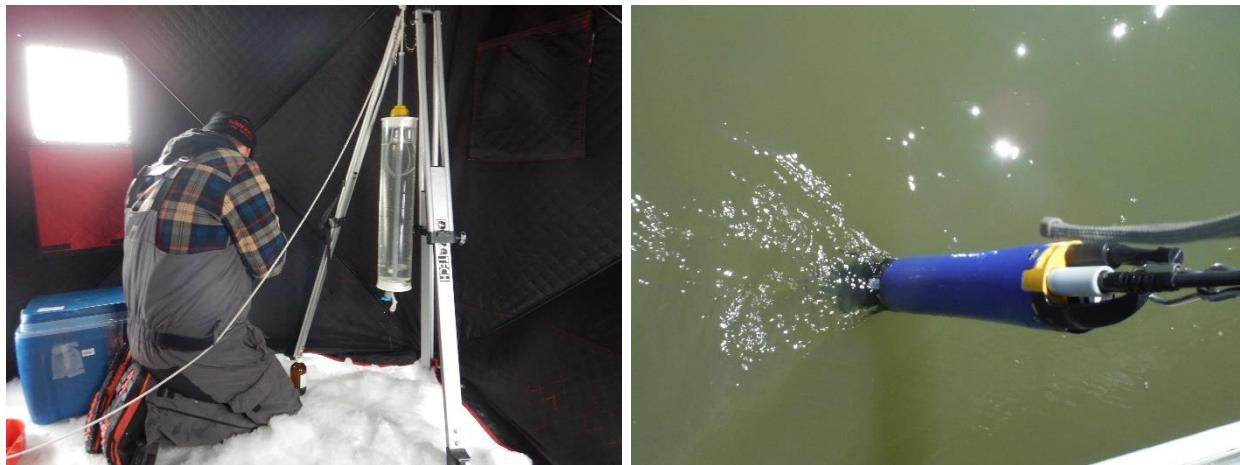
**Kemmerer water sampler (left) used to collect water at specific depths for laboratory analysis and water quality meter (right) used to measure on-site parameters (such as pH, dissolved oxygen, and temperature).**
