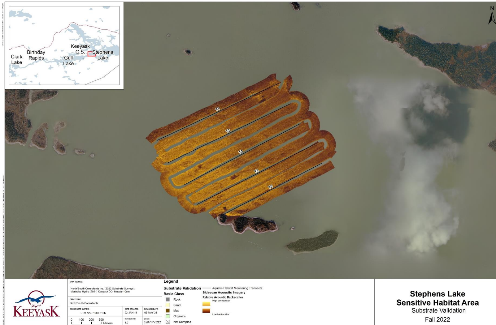
Map 15: Map illustrating the results of substrate composition sampling sites and acoustic imaging for the Stephens Lake sensitive habitat area, September 2022. Lighter colours in the acoustic imagery indicate harder substrates while darker colours indicate softer substrates.
