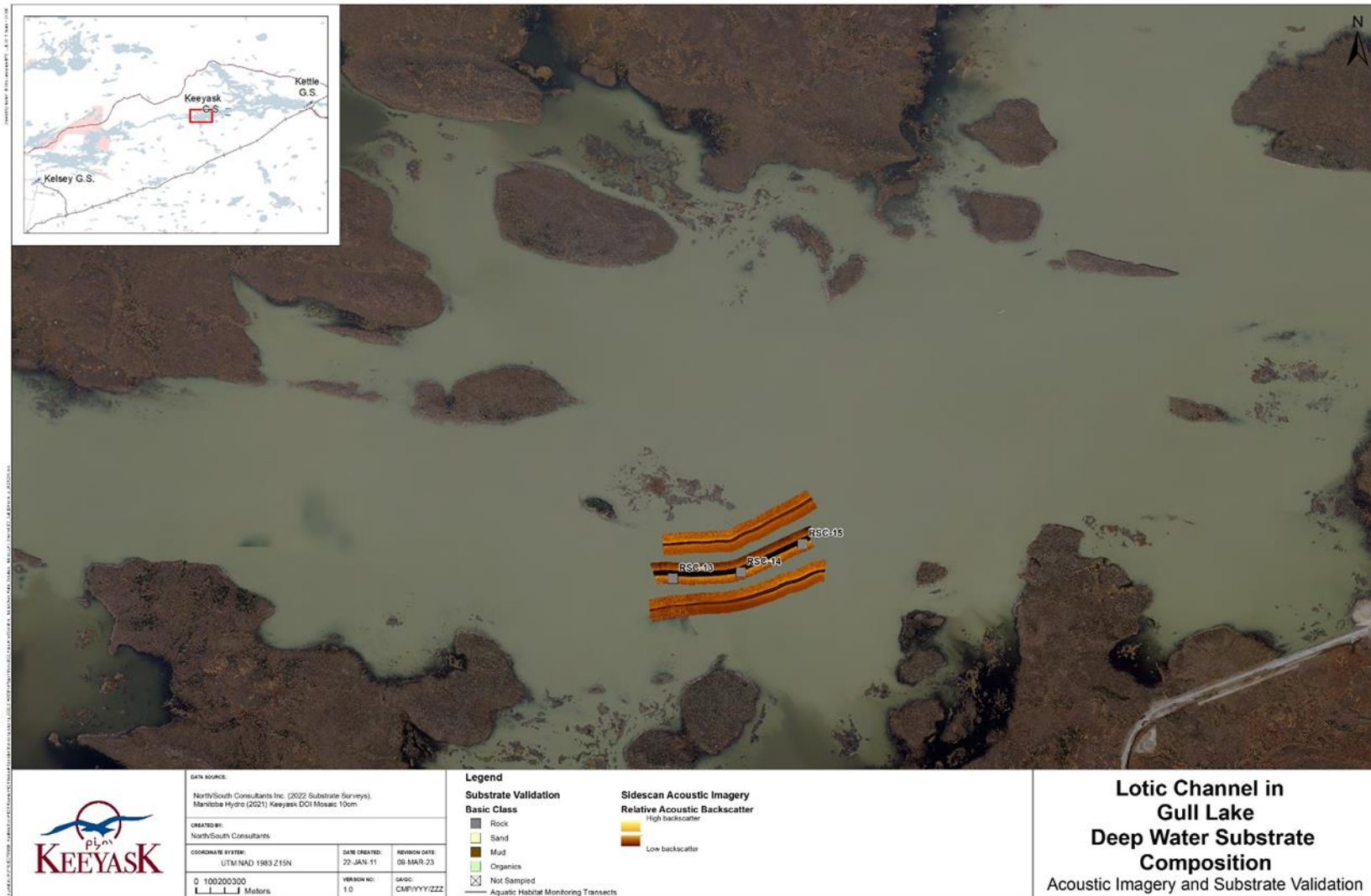
Map 9: Map illustrating the results of substrate composition sampling sites and acoustic imaging in the lotic portion of upper Gull Lake, 2022. Lighter colours in the acoustic imagery indicate harder substrates while darker colours indicate softer substrates.
