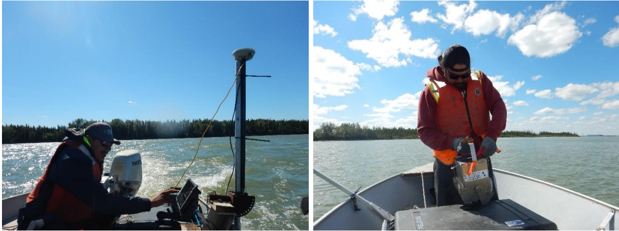
Setup of acoustic equipment (left) and Ponar dredge substrate sampler (right) used to monitor deep water and constructed habitats in the Keeyask reservoir and Stephens Lake in 2022.
