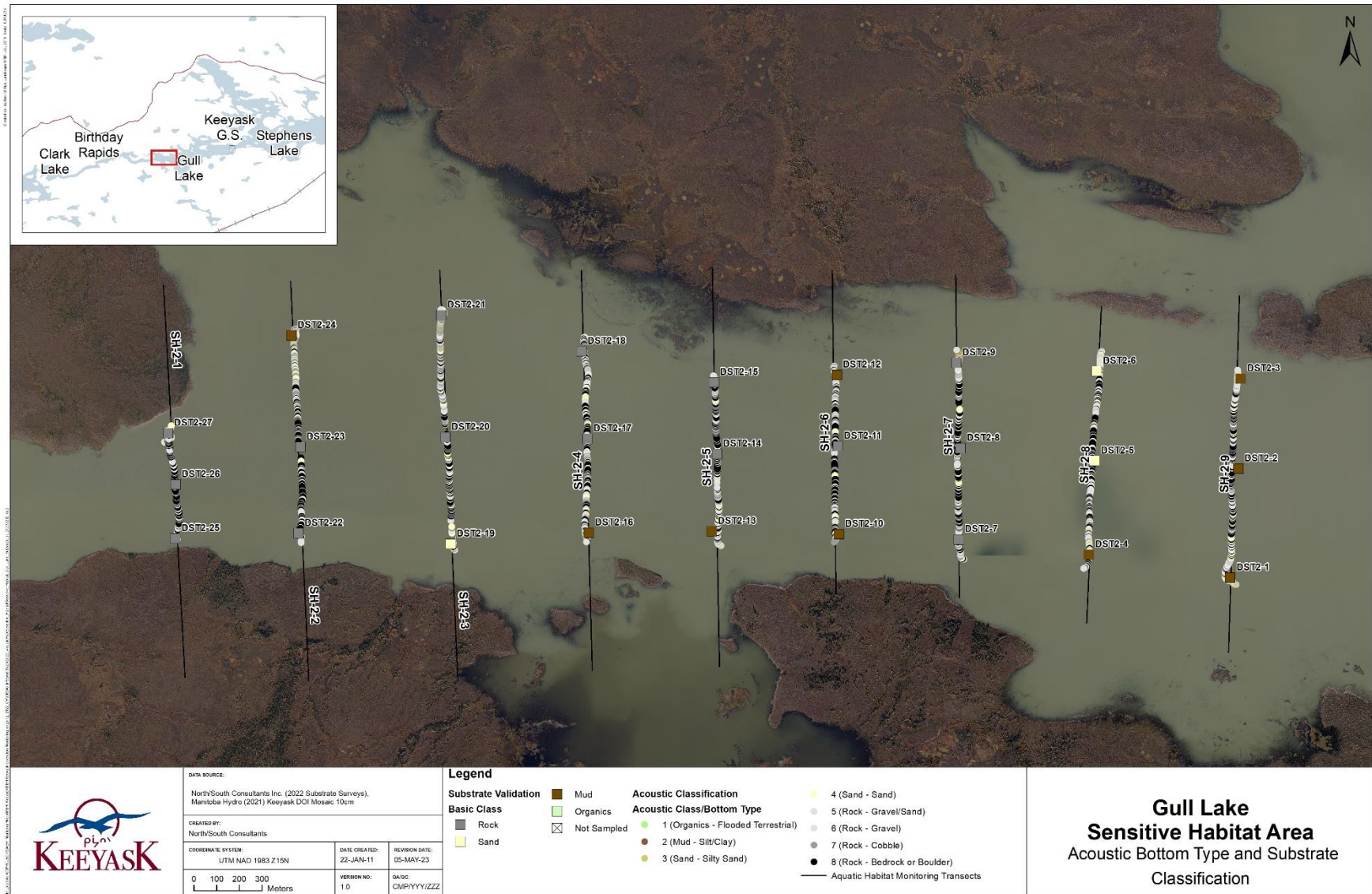
Map 8: Classified acoustic bottom type data and substrate validation results from substrate transect surveys conducted in the Keeyask reservoir at the Gull Lake entrance sensitive habitat area, 2022.
