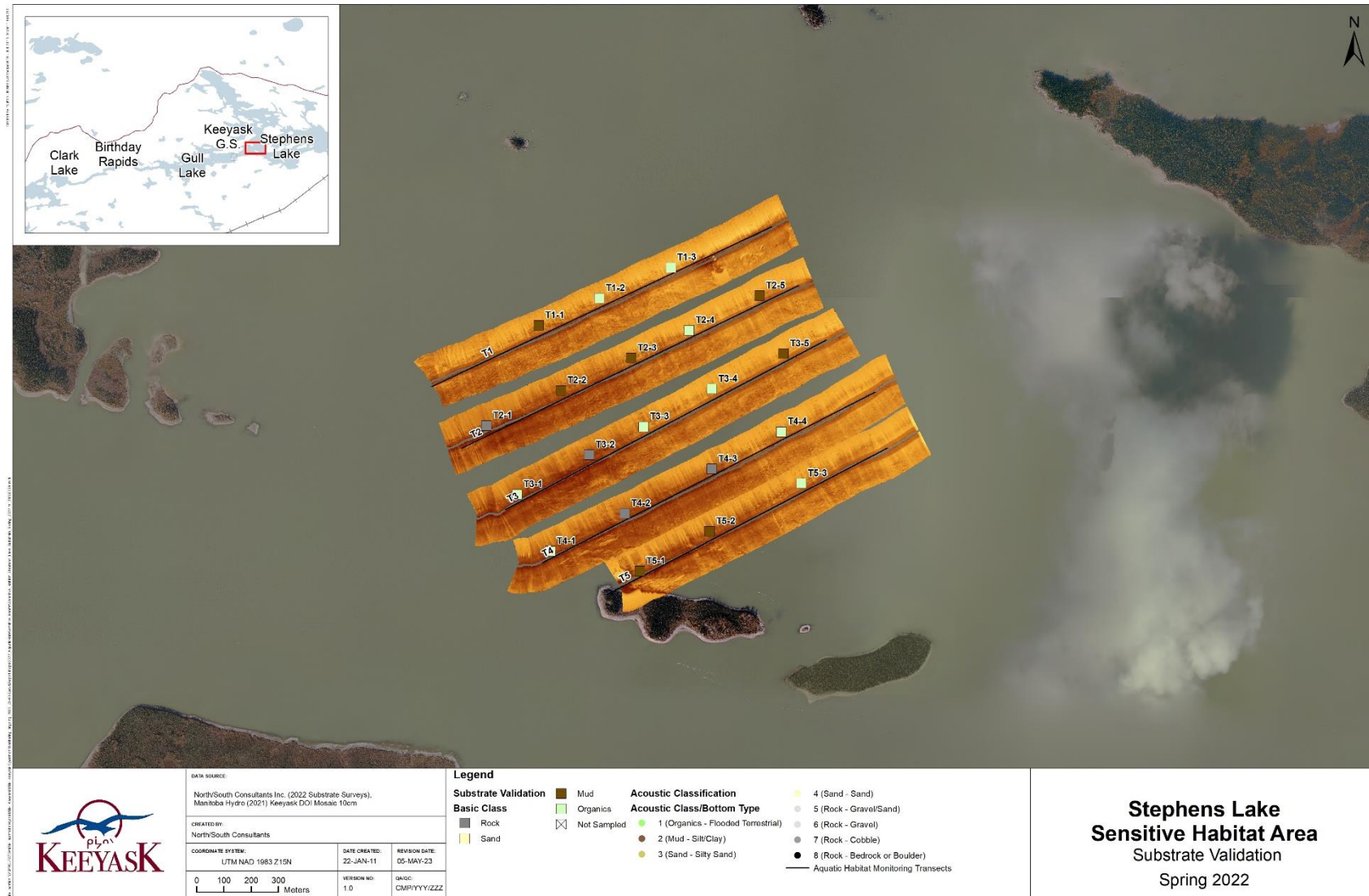
Map 13: Map illustrating the results of substrate composition sampling sites and acoustic imaging for the Stephens Lake sensitive habitat area, June 2022. Lighter colours in the acoustic imagery indicate harder substrates while darker colours indicate softer substrates.
