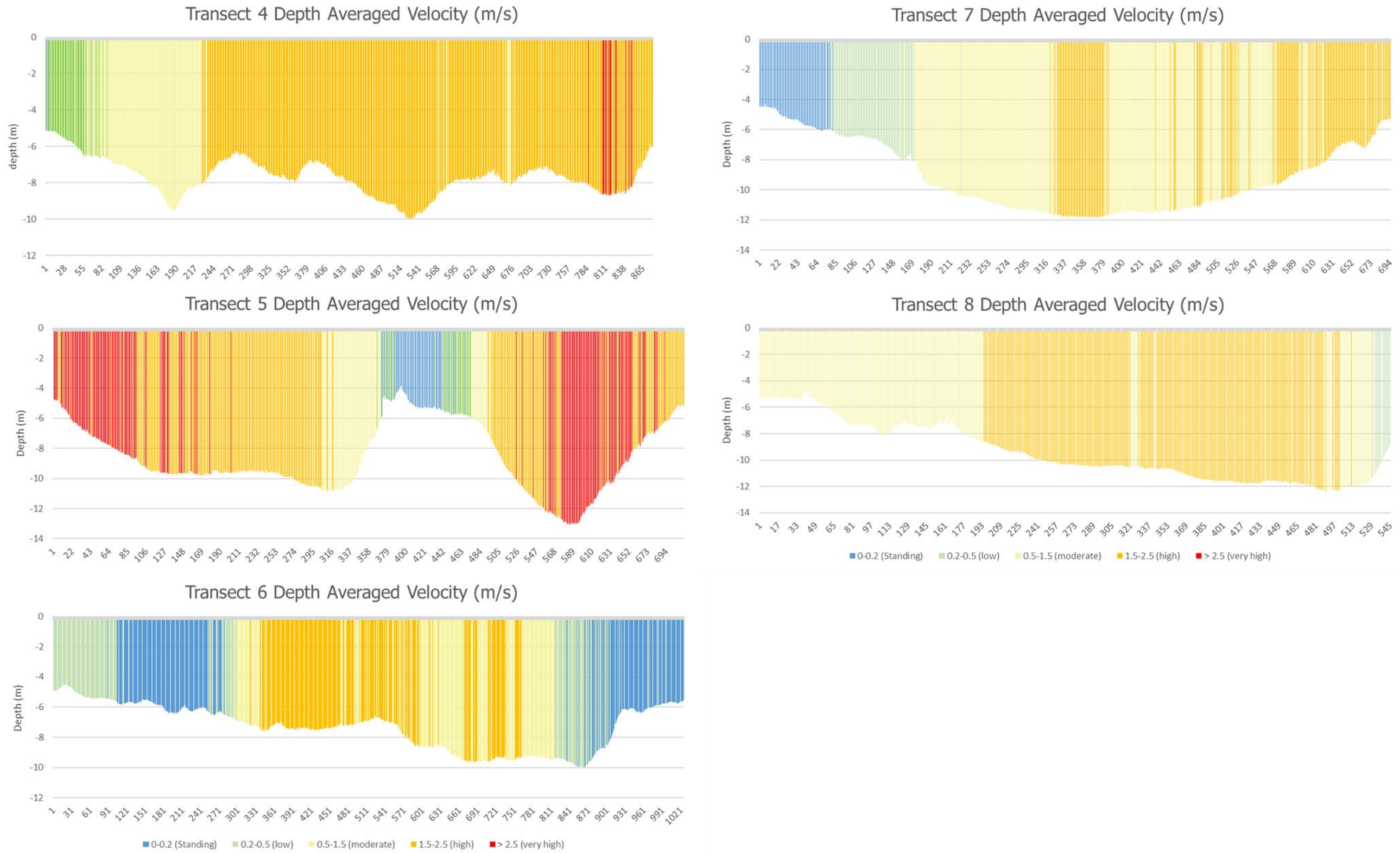
Figure 3: Classified sub-sampled depth averaged velocity representation of five transects sampled using an ADCP at the Birthday Rapids sensitive habitat area, 2022. Cross sections are viewed looking upstream (left to right bank).
