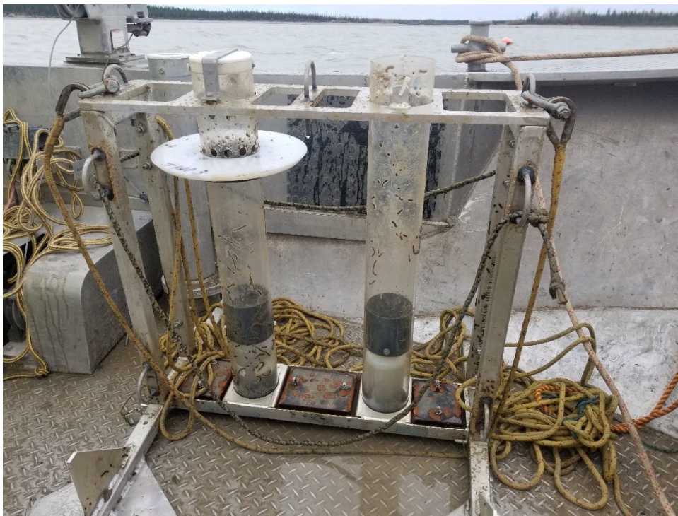
Photo 5: Sediment traps - 2 tube design
