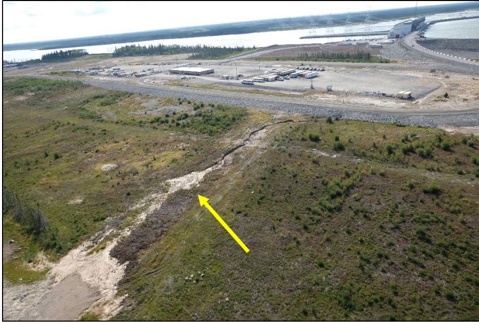
Photo 3-23: Runoff and sediment deposition (yellow arrow) along decommissioned road to EMPA D17-E in 2022
