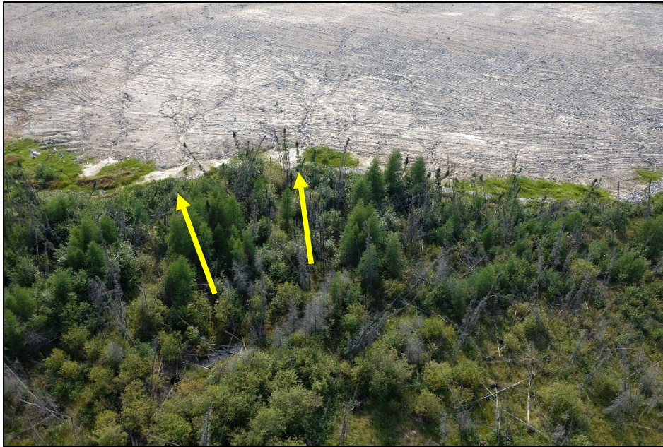
Photo 3-24: Sediment (yellow arrows) overtopping rock berm in EMPA D23(2)-E in 2022
