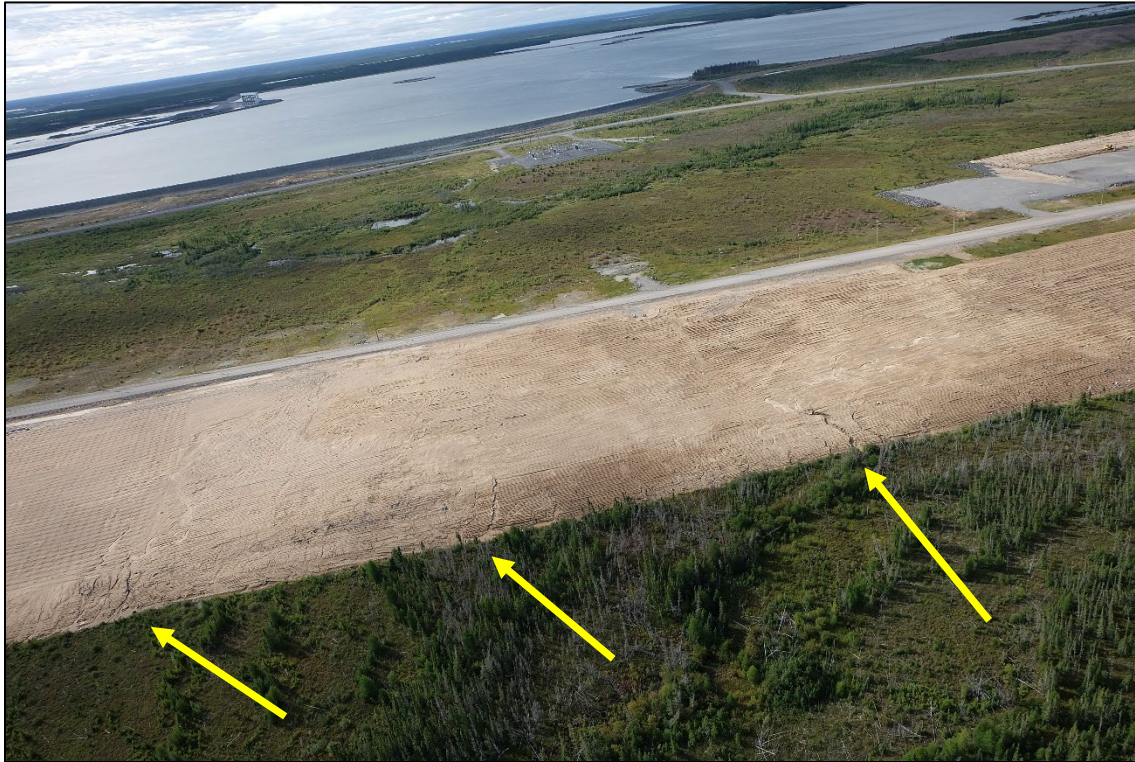
Photo 3-5: New locations where erosion may potentially cause sediment deposition into undisturbed vegetation (yellow arrows) along northern edge of Work Area A
