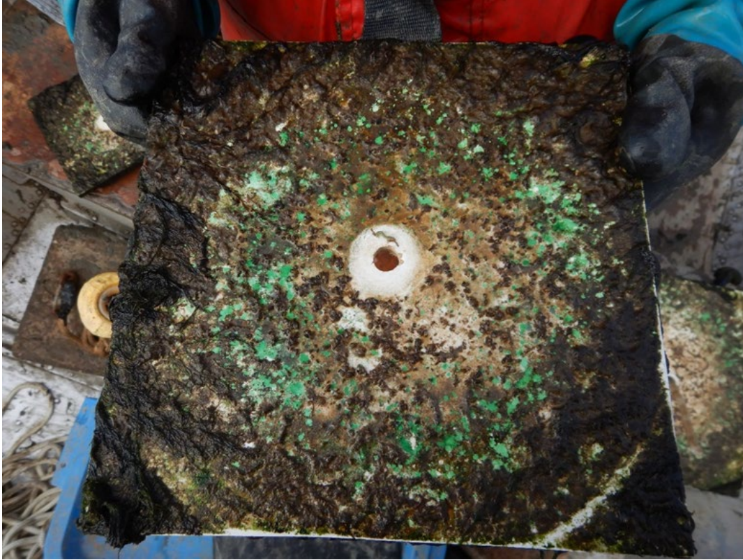
Figure 6: Adult zebra mussels attached to plate of a sampler at site ZM-09 at the end of the 2022 sampling period.
