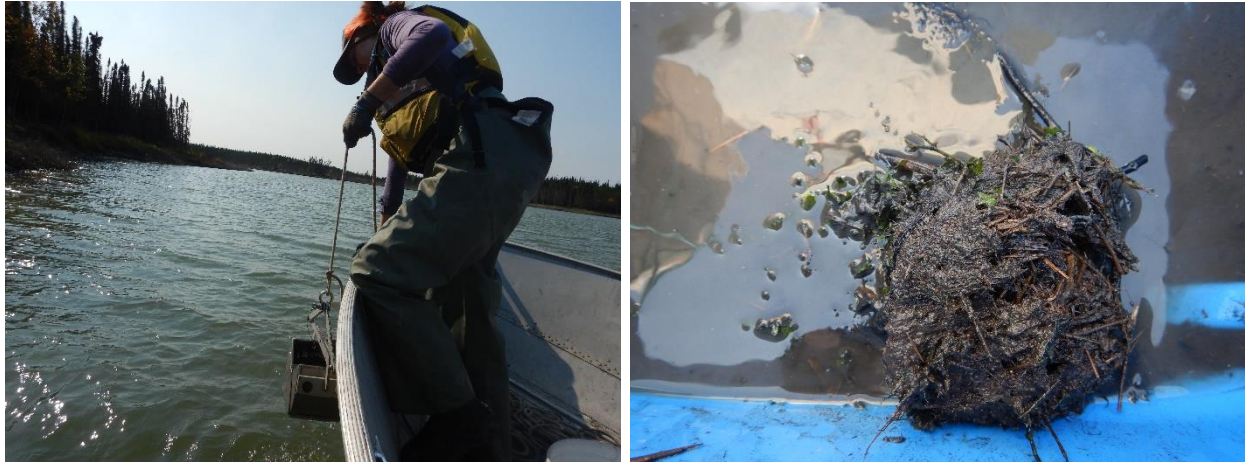
Collecting substrate (right) at a benthic invertebrate sampling site with a petite Ponar dredge (left) in the Keeyask reservoir, fall 2023.
