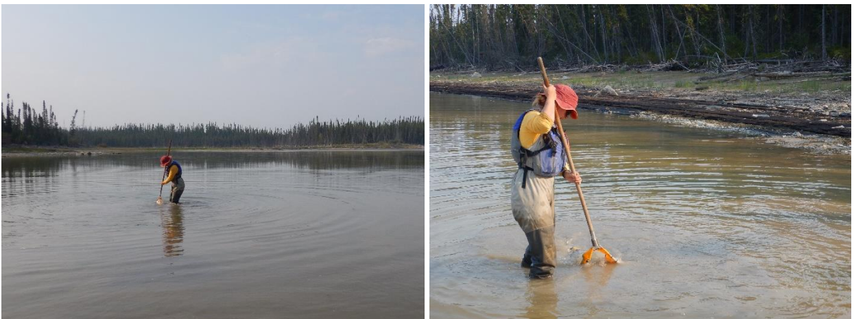
Using a kicknet to sample IE sites close to shore in Split Lake.
