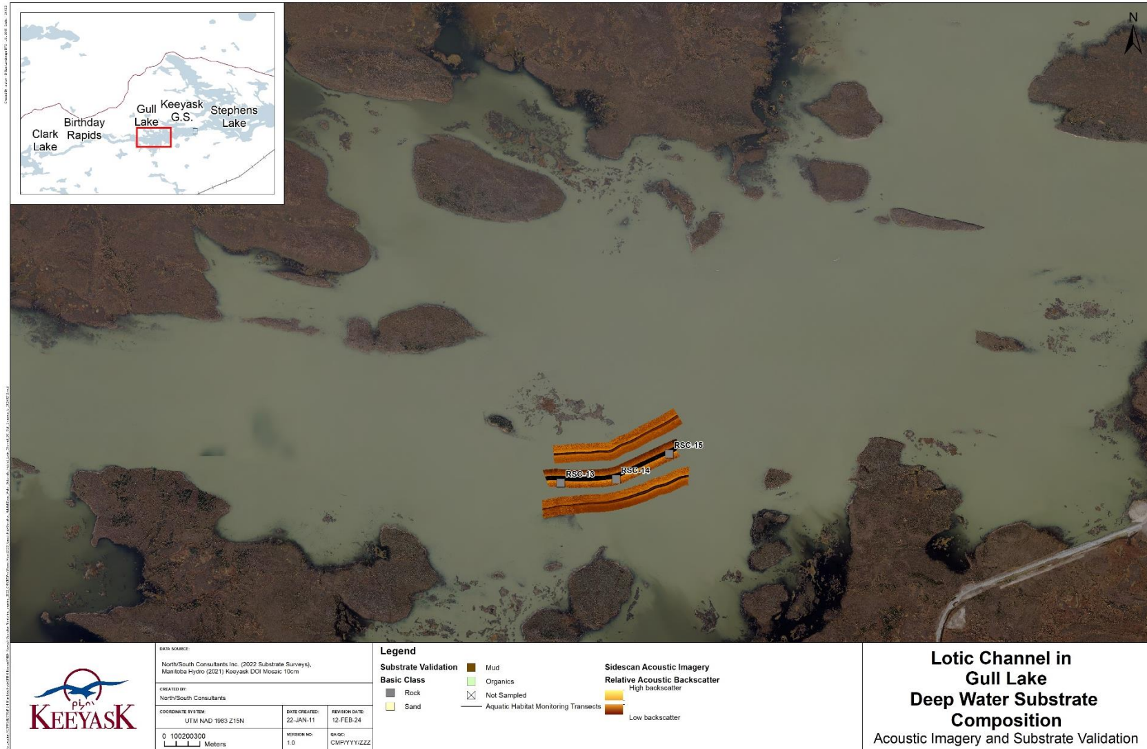
Map 9: Map illustrating the results of substrate composition sampling sites and acoustic imaging in the lotic portion of upper Gull Lake, 2023. Lighter colours in the acoustic imagery indicate harder substrates while darker colours indicate softer substrates.
