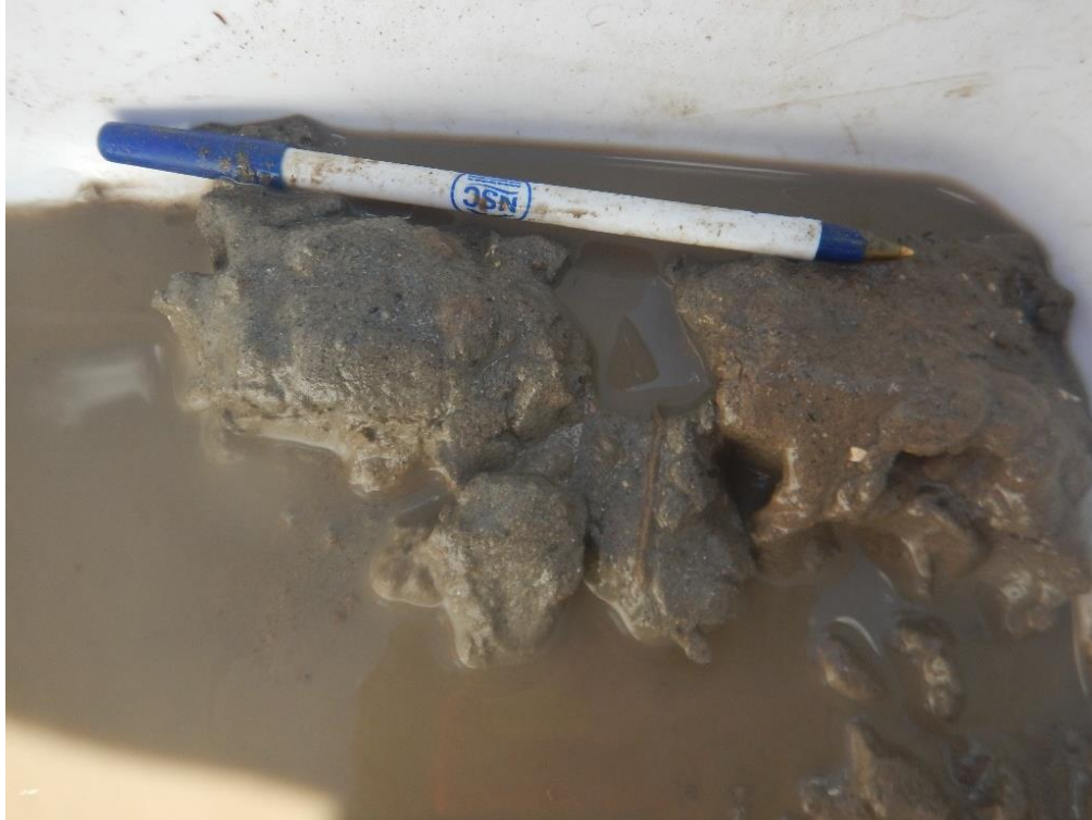
Photo 3: Substrate collected at site DST4-3 in the upper Stephens Lake sensitive habitat area in August showing sand and clay.
