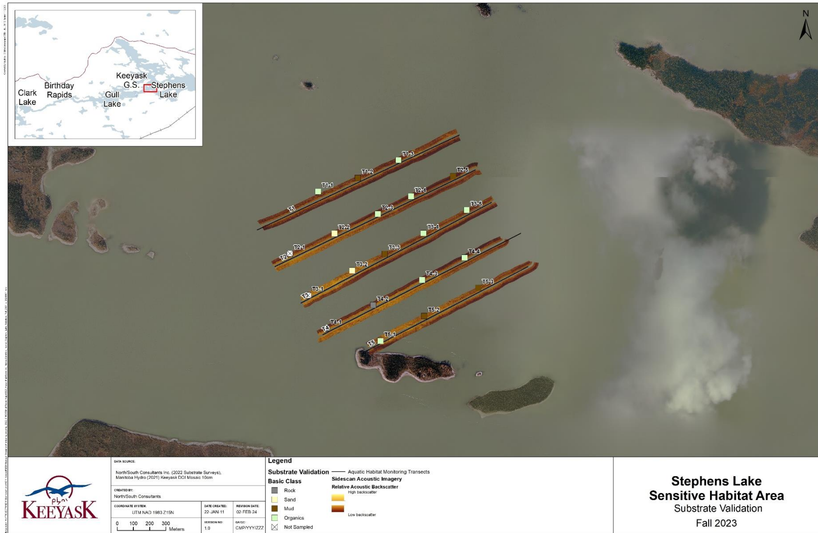
Map 15: Map illustrating the results of substrate composition sampling sites and acoustic imaging for the Stephens Lake sensitive habitat area, September 2023. Lighter colours in the acoustic imagery indicate harder substrates while darker colours indicate softer substrates.
