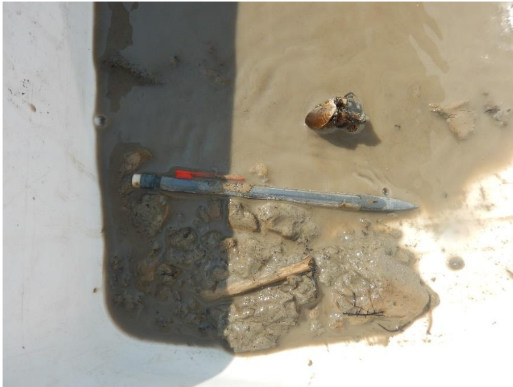
Photo 7: Substrates collected from constructed shoal G-North-2 in the Keeyask reservoir, showing clay and silt and collected zebra mussels, 2023.
