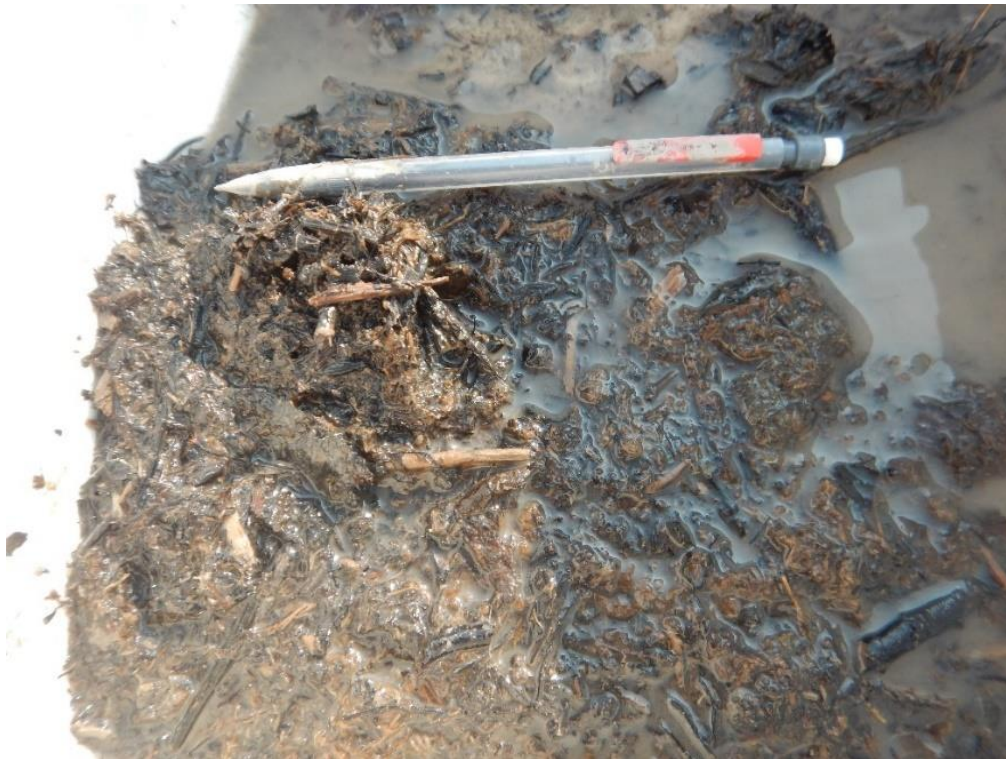
Photo 9: Substrates collected from constructed shoal H-North-4 in the Keeyask reservoir, showing organics and silt.
