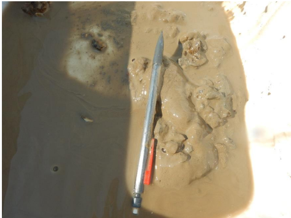
Photo 6: Substrates collected from constructed shoal F-South-3 in the Keeyask reservoir, showing clay and silt, 2023.
