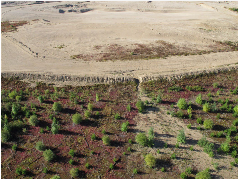
Photo 2-3: Identifying an area with sedimentation from a Project borrow area into the surrounding native habitat during an aerial survey
