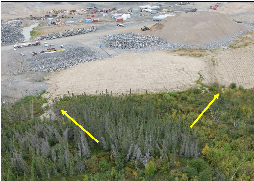
Photo 2-21: Example of an area with sediment deposition into priority habitat (Tall shrub vegetation on thin peatland site) in September, 2021
