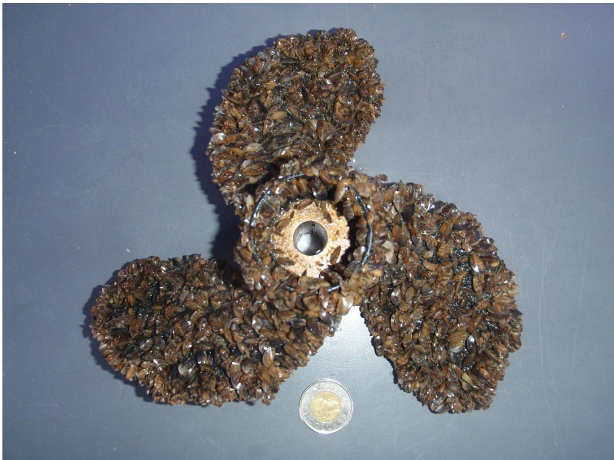
Figure 1: Once present, zebra mussels grow on hard surfaces that are in the water, as shown on this boat propeller. Each mussel is approximately the size of a fingernail.
