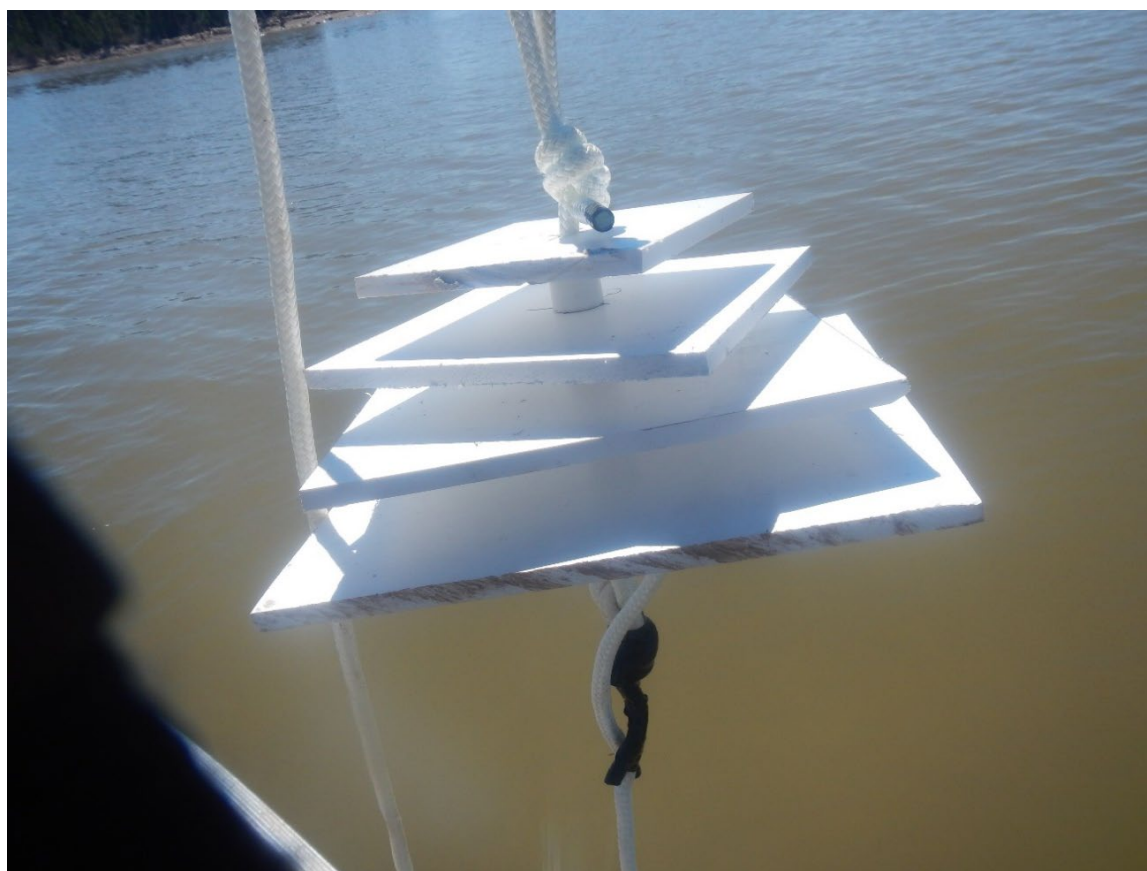
Figure 3: Adult zebra mussel sampler set in the Keeyask area, 2023.
